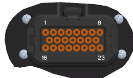
DETAIL B TYCO/AMP 23 PIN PART # 776228-1 SCALE 0.500
