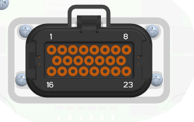
DETAIL D TYCO/AMP 23 PIN PART # 776228-1 SCALE 0.500
