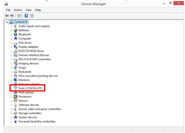
• With Ports highlighted use the right arrow key to expand this menu option. Then hit the down arrow key until the *USB Serial Port (COM4)* is highlighted. With it highlighted press the enter key to open its settings.
